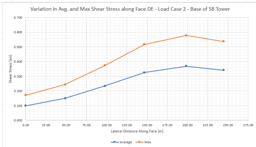
Figure 11: Shear Stress Distribution Along Plane DE for ISA Governing STR III Load Combination
