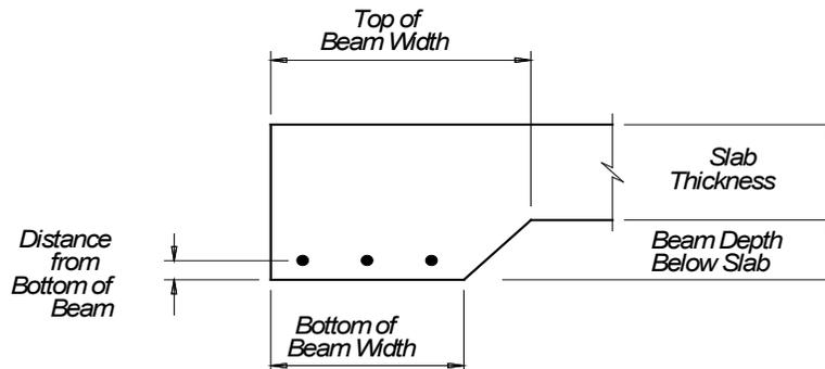
*Figure 9. Flat Slab Beams.*
