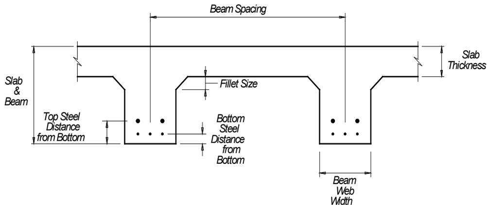
Figure 4. T-Beam Diagram.
