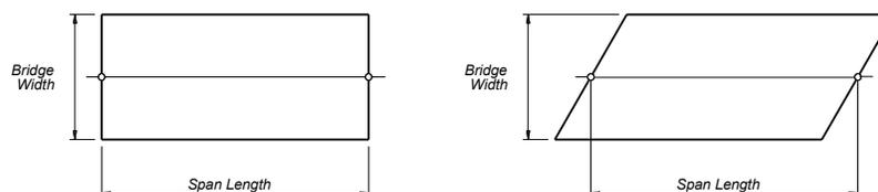
Figure 6. Flat Slab Geometry.
