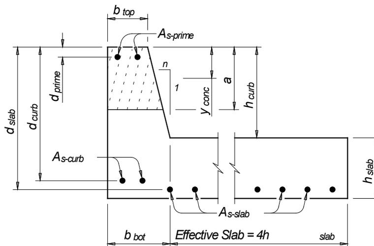
Figure 16. Curb for Flat Slab Bridges.
